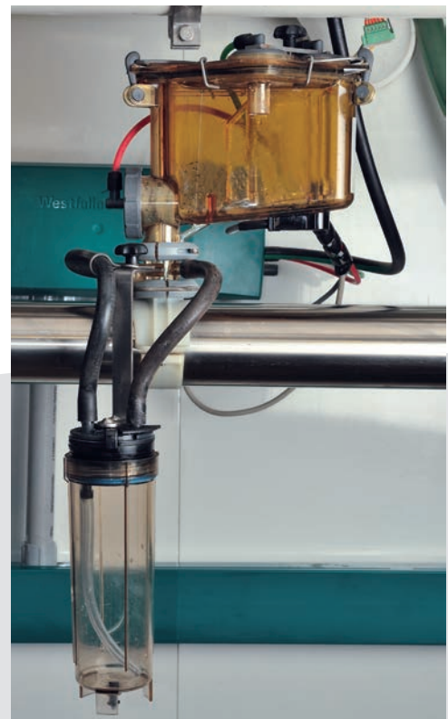
Optional butterfat sampler on DemaTron 70 and DemaTron 75.
